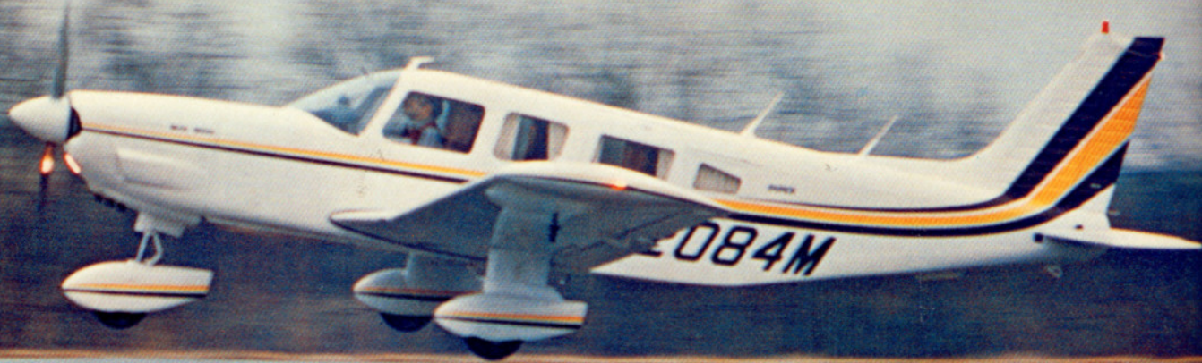
The craft's long snout comes high on landings. Redesigned wheel and strut fairings are apparent. Photos by Roger Rozelle.
