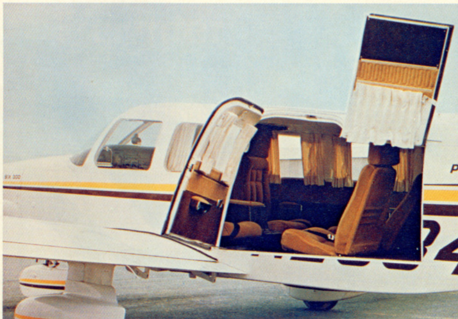
By opening rear cabin and baggage doors together, a large entryway is created. Club seating arrangement calls for intertwining legs of front- and rear-facing passengers.
