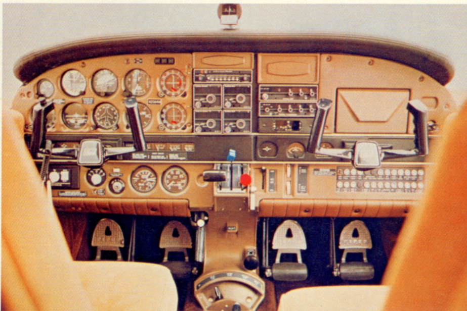
The Six's panel comes from the same mold as that of other Cherokees. However, five rocker switches have been moved from in front of the throttle to the left sidewall.
